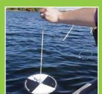
The Secchi disk created in 1865 by Angelo Secchi—is a circular disk used to measure water transparency. The depth at which the pattern on the disk is no longer visible is taken as a measure of
